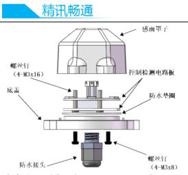
(1) Assembly the sensor according to the figure above and pull the waterproof washers several times during installation so that it can easily fit. Apply some waterproof silicone grease to the waterproof washers and screws.
