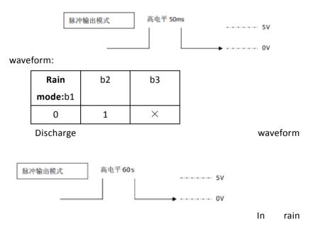
sensing mode, an effective pulse was output for 1 minute for about 0.05ml raindrops perceived. After 1 minute, every 10 seconds, if a rain drop is detected, otherwise the output was terminated.
