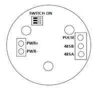
The SWITCH ON position in the figure is the dial-up switch position, which represents the b3, b2, b1. from top to bottom The operating mode of the rainfall sensor can be selected, as well as the output function.
