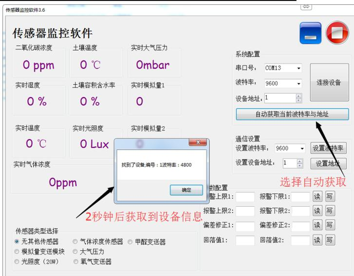
Then click the connected device to get the sensor data information in real time.
