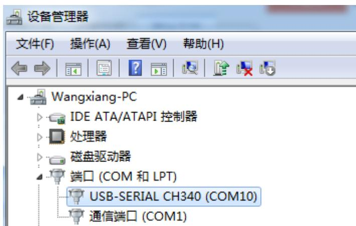
As shown in the figure above, your serial number is COM10 at this time, please remember this serial port, you need to fill in this serial number in the sensor monitoring software.
