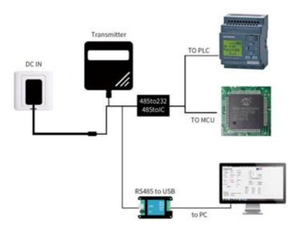
This product can also be used by multiple sensors combined in a 485 bus. In theory, one bus can connect more than 16 485 sensors. If more 485 sensors are needed, more 485 devices can be expanded using 485 repeaters. The other end is
