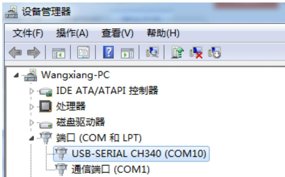
As shown in the figure above, your serial number is COM10 at this time, please remember this serial port, you need to fill in this serial number in the sensor monitoring software.
