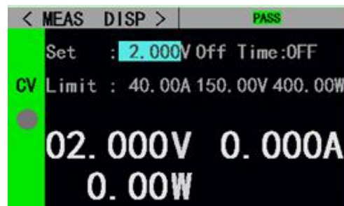
Figure 2.14.2 Interface displayed when the qualification test is being started
