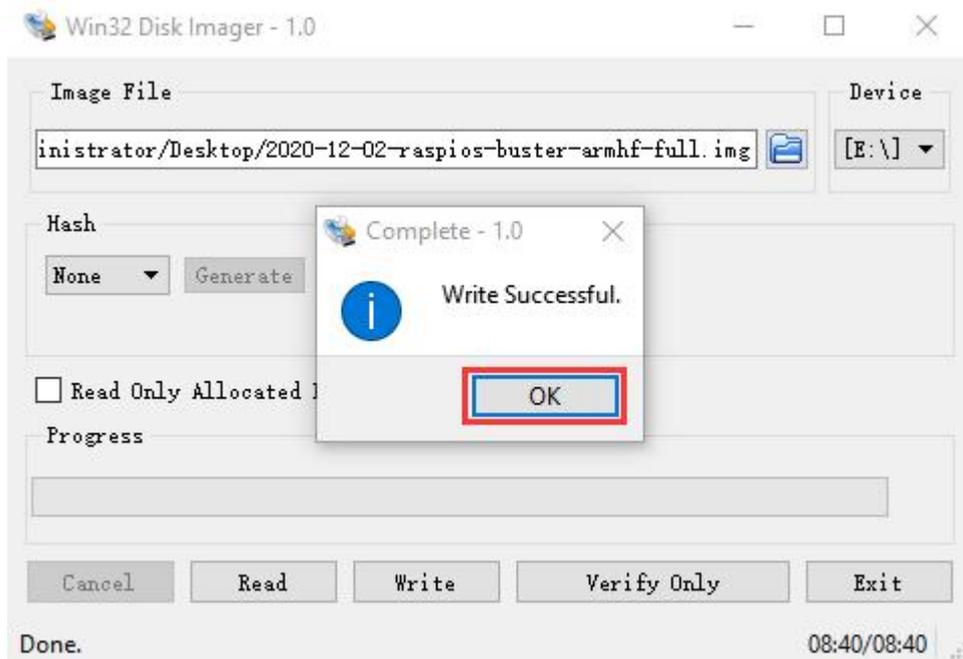
Don' t eject card reader after burning mirror system, build a file named SSH, then delete .txt.
