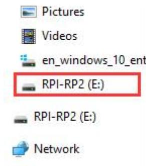
Move the UF2 file into "RPI-RP2" , and the Raspberry Pi Pico will automatically restart. At this point, the burning is complete.
