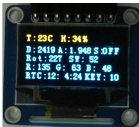
Figure 7: OLED displays relative sensor parameters
